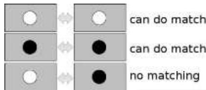
Fig 3: Matching of blobs on the basis of Contrast in SURF
