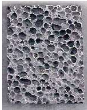
Figure 1: valid porosity varied from 80 to 85% of aluminium alloy foams
