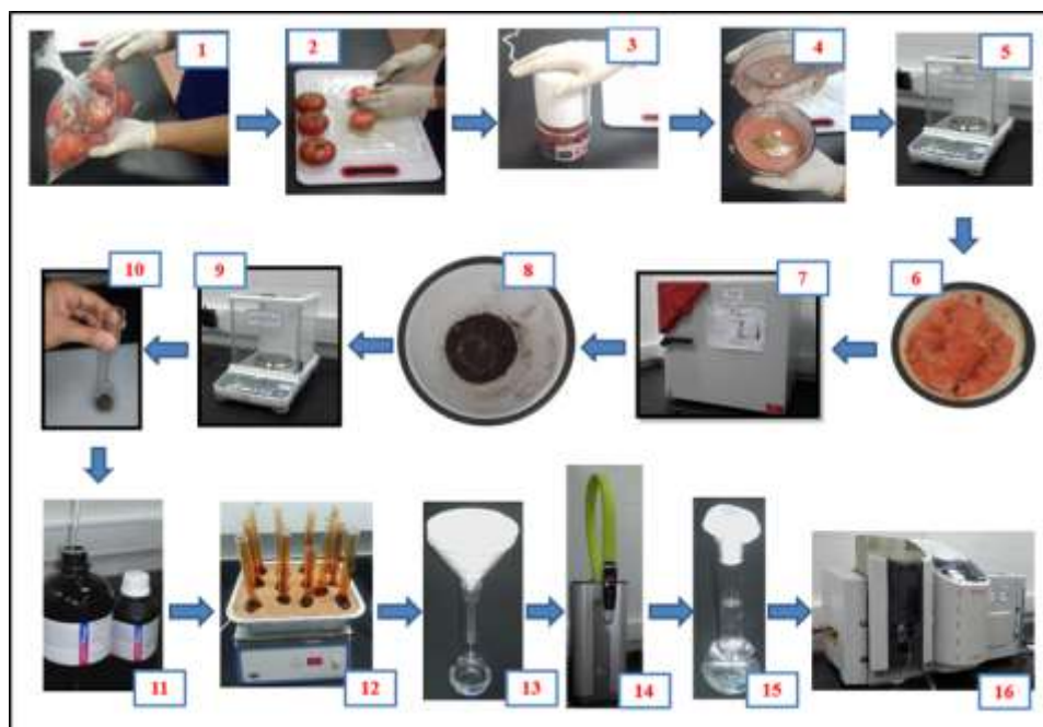
Fig. 2: Schematic diagram of the determination of heavy metals in tomato using FAAS
