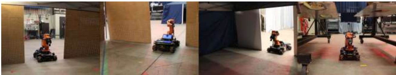
Fig. 5: The robot entering the illuminated enclosure, exiting the illuminated enclosure, entering the unlit enclosure, and traversing under the pair of wing sections.
