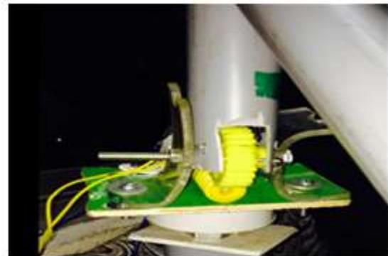
Fig 1.2: Spur Gear and Worm gear coupled
