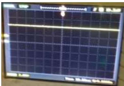
Fig.21. Output Voltage of Solar panel
