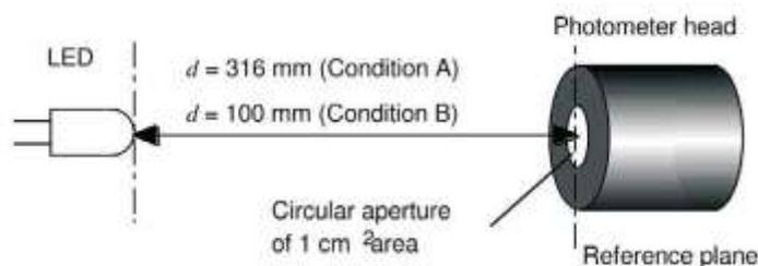
Fig 3: Geometry for CIE averaged LED intensity
