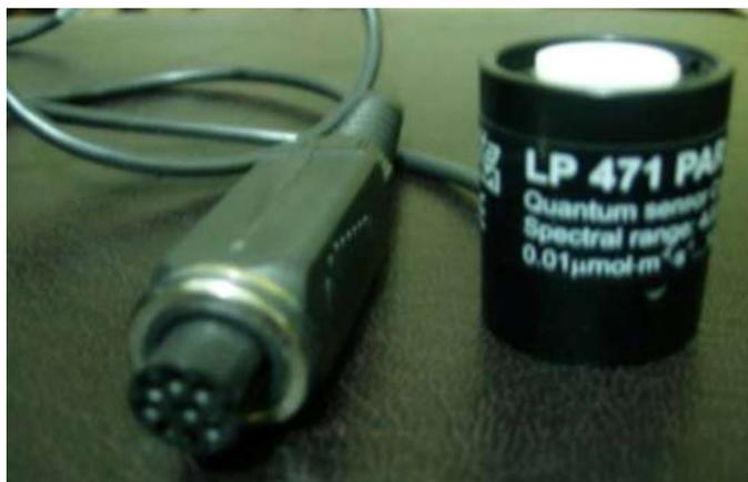
Fig 2: Photosynthetic active radiation sensor (LP 471PHOTO, DELTA OHM)
