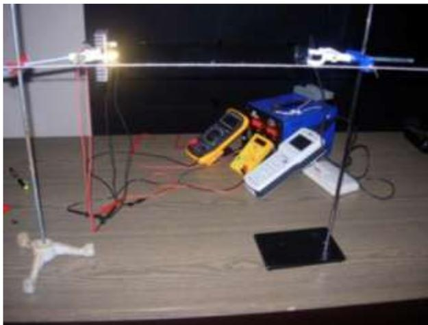
Fig 1: Test method used to determine the PAR values of the LEDs
