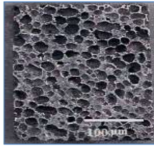
Figure 1: porosity varied from 76 to 88% of AAF
