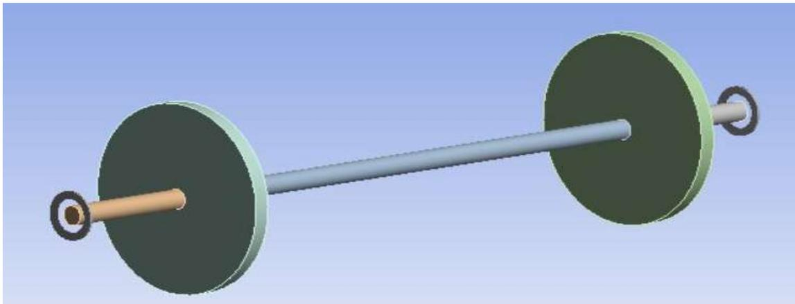
Fig. 3: Model of the rotor studied in ANSYS Workbench.
