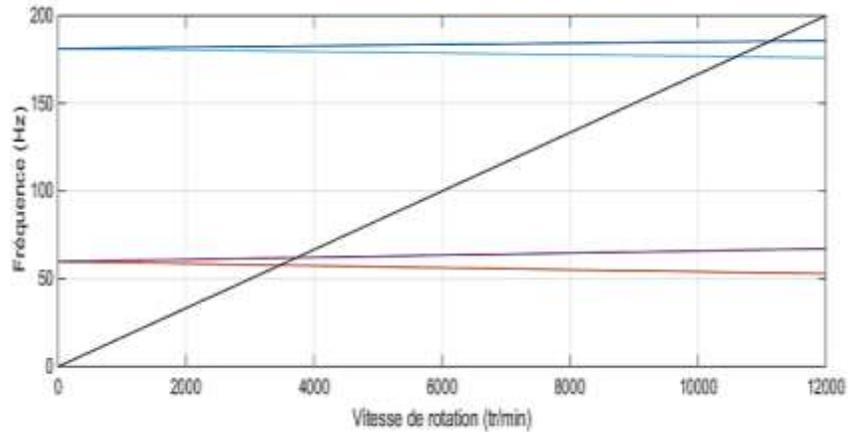
Fig. 5: Campbell diagram of uncracked rotor generated by our program of MATLAB.
