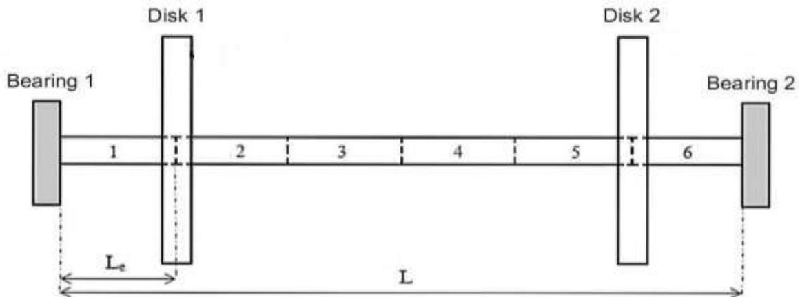
Fig. 2: Finite element model of the rotor studied.
