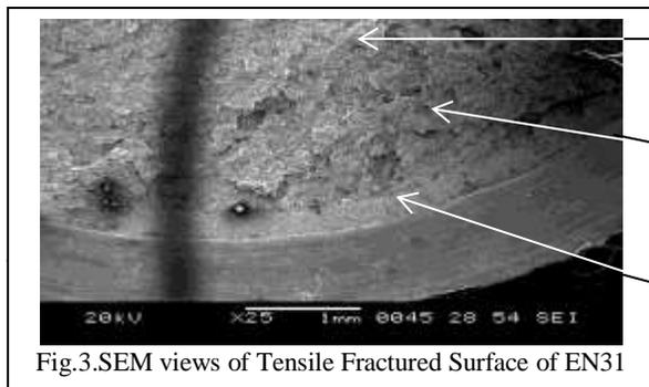
Fig.3.SEM views of Tensile Fractured Surface of EN31
