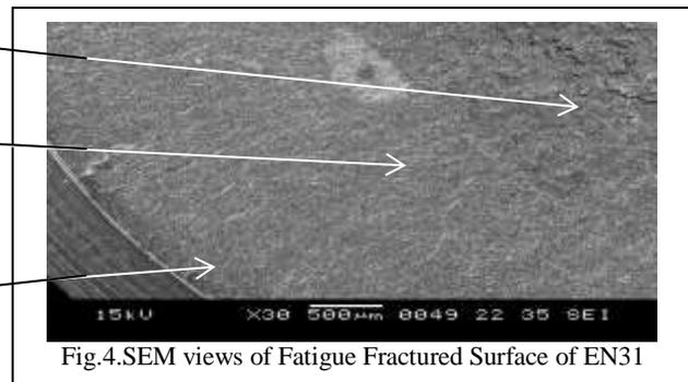
Fig.4.SEM views of Fatigue Fractured Surface of EN31
