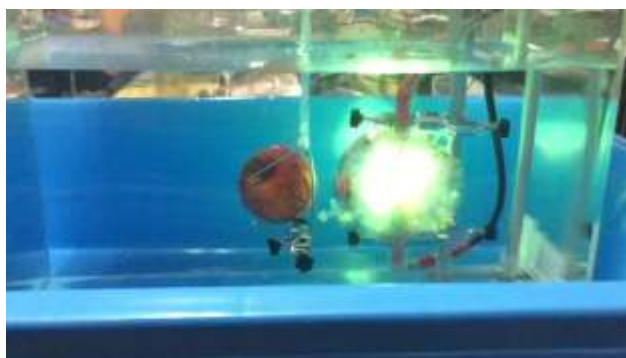
Fig. 3: Discharge process in the non-thermal food processing system utilizing an underwater shockwave.
