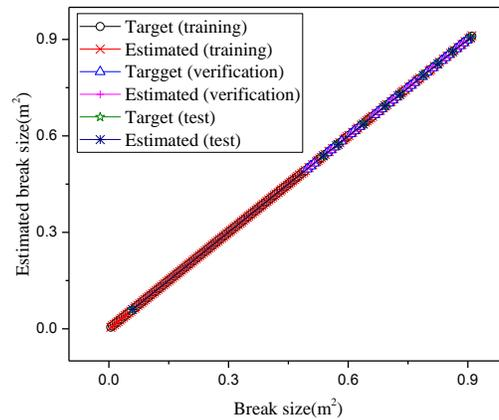
Fig. 7: Target breaks sizes and estimated break size (cold-leg LOCA)
