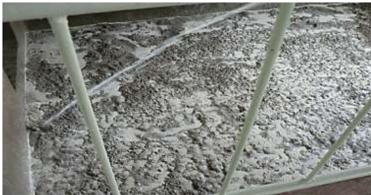
Fig. 2: Spraying the solution on quartz sand filter
