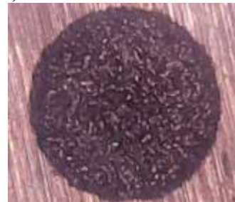
Fig. 4: Influence of peak current on EDMed surface using a) I = 25A and b) I = 10A
