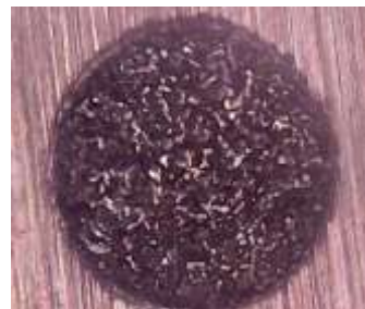
Fig. 4: Influence of peak current on EDMed surface using a) I = 25A and b) I = 10A
