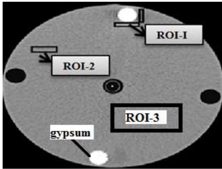
Fig. 2: Regions of interest: ROIs-1 and ROI-2 were used for beam hardening artifact assessment. ROI-3 ( $400 \text{ mm}^2$ ) was used to measure the standard deviation (Image noise measurements).
