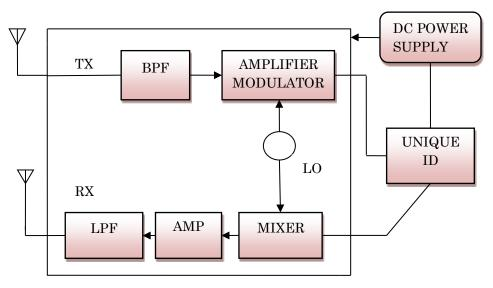
Fig.1. Block diagram of UHF Active tag
