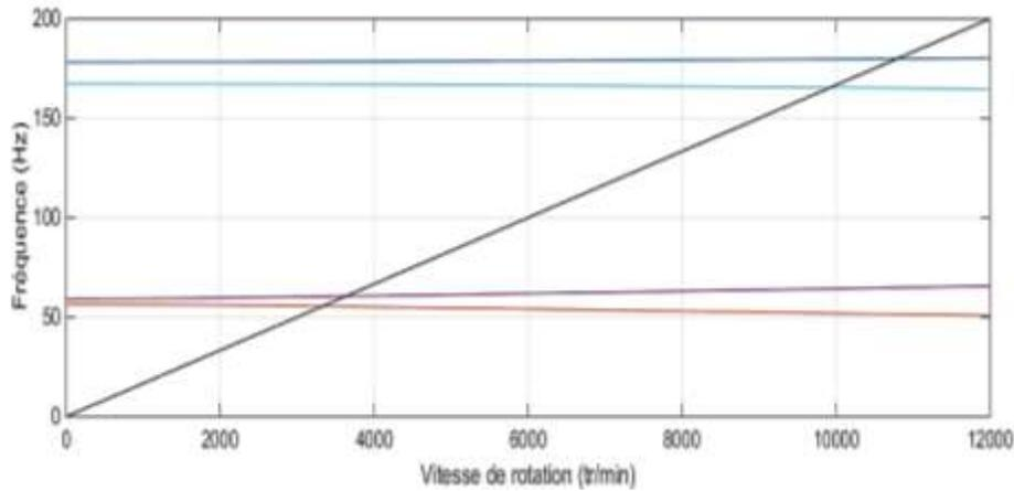
Fig. 7: Campbell diagram of uncracked rotor generate by our program of MATLAB where the crack is located in 0.14 m from the left bearing and  $\mu=0.46$ .
