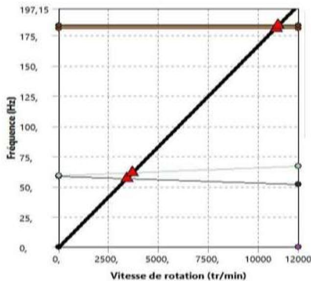
Fig. 6: Campbell diagram of cracked rotor generate by ANSYS Workbench where the crack is located in 0.14 m from the left bearing and  $\mu=0.46$ .
