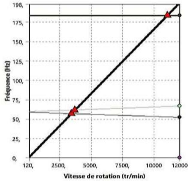
Fig. 4: Campbell diagram of uncracked rotor generated by ANSYS Workbench.
