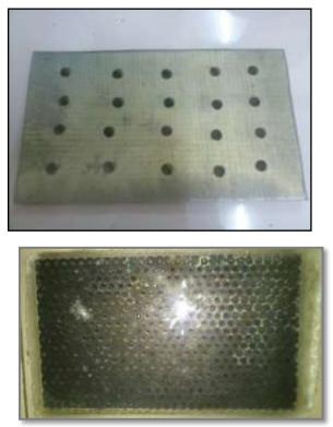
Fig. 2a & b: Hybrid aluminum (upper) and hybrid steel (below)material.
