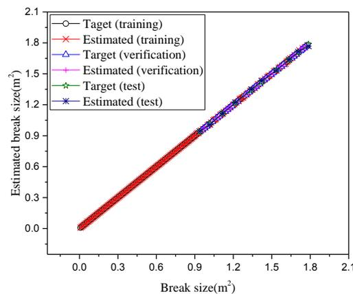
Fig. 6: Target break sizes and estimated break size (hot-leg LOCA)
