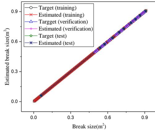
Fig. 7: Target breaks sizes and estimated break size (cold-leg LOCA)
