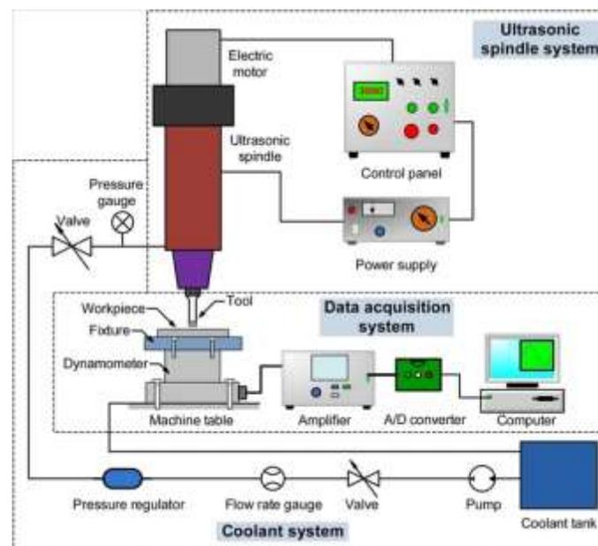
Fig. 1: Experimental set-up on a RUM
