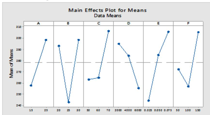
Fig. 4: Main effect plot for Equivalent Cutting force
